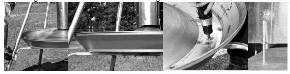
8. To install the Lid, remove the Self-Tapping Screw from the Elbow Bracket on the Lid and insert the Lid Arm into the bracket, using a Rubber Hammer to tap it in. On the side of the Hopper, remove the Bolts / Wing Nuts from the handle brackets. Put the Lid on top of the Hopper, with the handle pointing away from where the Control Box is located, while fitting the Lid Arm
