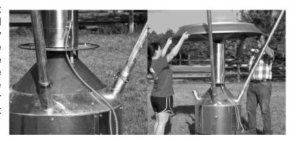
3. Find the four Stabilizer Rods in the Hardware Bag. Rotate the Trough on top of the Motor Shaft until all 4 holes line up with the Bolt / Washer sets near the top of the Shaft.
