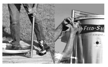
in the brackets on the side panel. Make sure the Lid seats completely in place, and re-attach the Bolts / Wing Nuts. Tighten Wing Nuts snuggly, while still allowing the handle to move up and down easily. Once you have the Handle pointing parallel to the side panel of the Hopper, use your Cordless Drill to re-install the Self-Tapping screw at the top in the Elbow Bracket, and tighten the bolts in the Lid Elbow.
