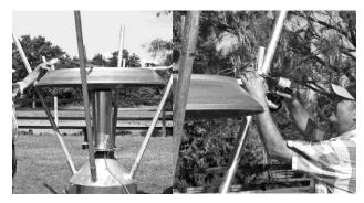
5. Tighten the Leg Sleeve bolts completely, using the 1/2 inch wrench, securing the Legs to the Hopper.
