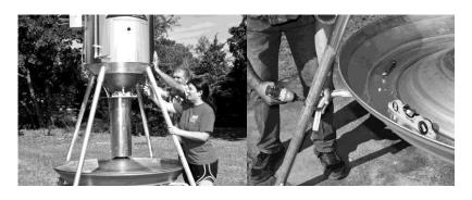
Clamps (where needed) so legs can slide up or down to complete the leveling procedure. When finished with each, check that all Bolts and Screw Clamps are tightened completely. After filling your feeder's hopper, you should hear a "CLANK" sound when you close the lid. Check around it, to be certain it isn't hung up on one of the bolt heads. Improper lid closure could result in wet feed.
