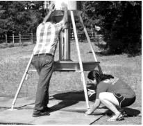
7. Loosen all Screw Clamps at Legs and push the Feed Trough down until it hangs from the Stabilizer Rods, equally all around. Position the 4-Way Trough Support Assembly so that it just touches the Trough bottom and tighten the Screw Clamps. Attach the Feed Trough to the Trough Support Assembly using the 4 remaining Self-Tapping Screws, putting each near the middle of the Trough bottom. It's now time to tighten the Bolt / Washer sets holding the Stabilizer Rods in the Motor Shaft.
